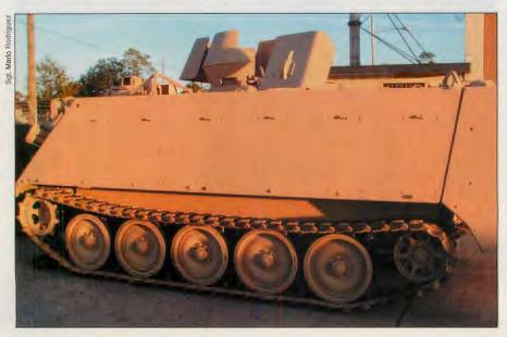
A proven idea on a proven vehicle is the ACAV-type armor being added to the M113series vehicles.
